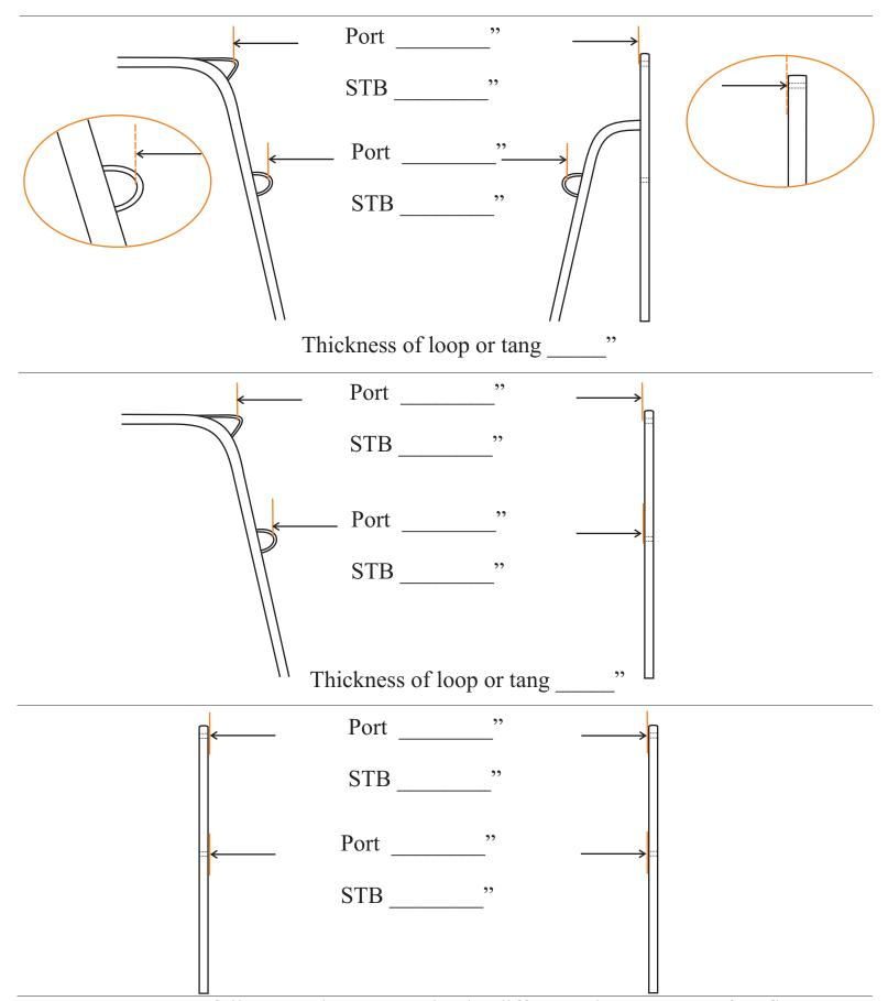
Measure very carefully, as a 1/16" can make the difference between a perfect fit or a struggle to fit. This is particularly true when measuring for both uppers and lowers. So measure twice or even thrice!
